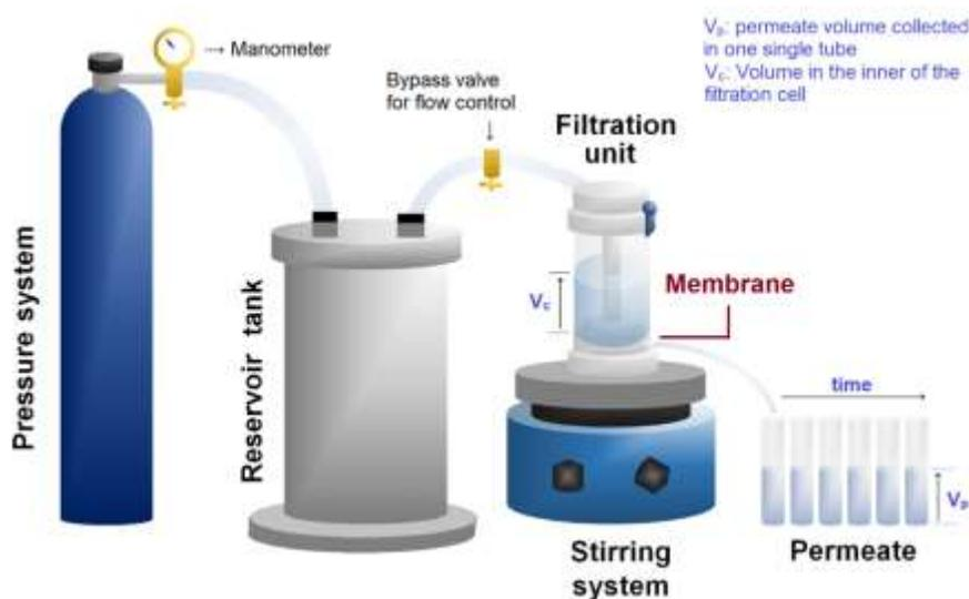
**Figure 1.** Schematic representation of inert system components by dead-end ultrafiltration.
